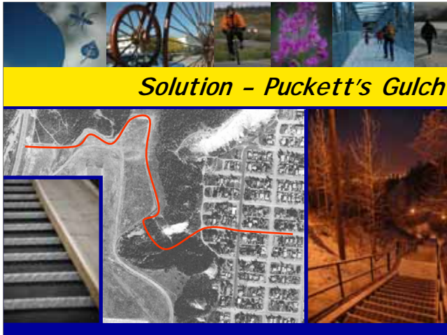
Stairs following Edmonton standards with a bike ramp along one side 50 m climb = 275 steps
