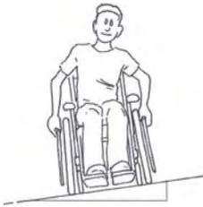
**PROBLEM** Wheelchair users traveling on a sidewalk with a cross slope greater than 2% use more energy to to offset the force of gravity that directs them towards the curb and into the street
